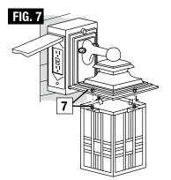
This fixture has a photocell light control located on the front of the canopy. Wall switch should always be on. The LED lights will turn on when the ambient light around diminishes to a nighttime light level. The lights will remain on until the ambient light has risen back to daylight level. Avoid installing the fixture near nighttime light sources, such as streetlights or other light fixtures, which might prevent the light from turning on.
